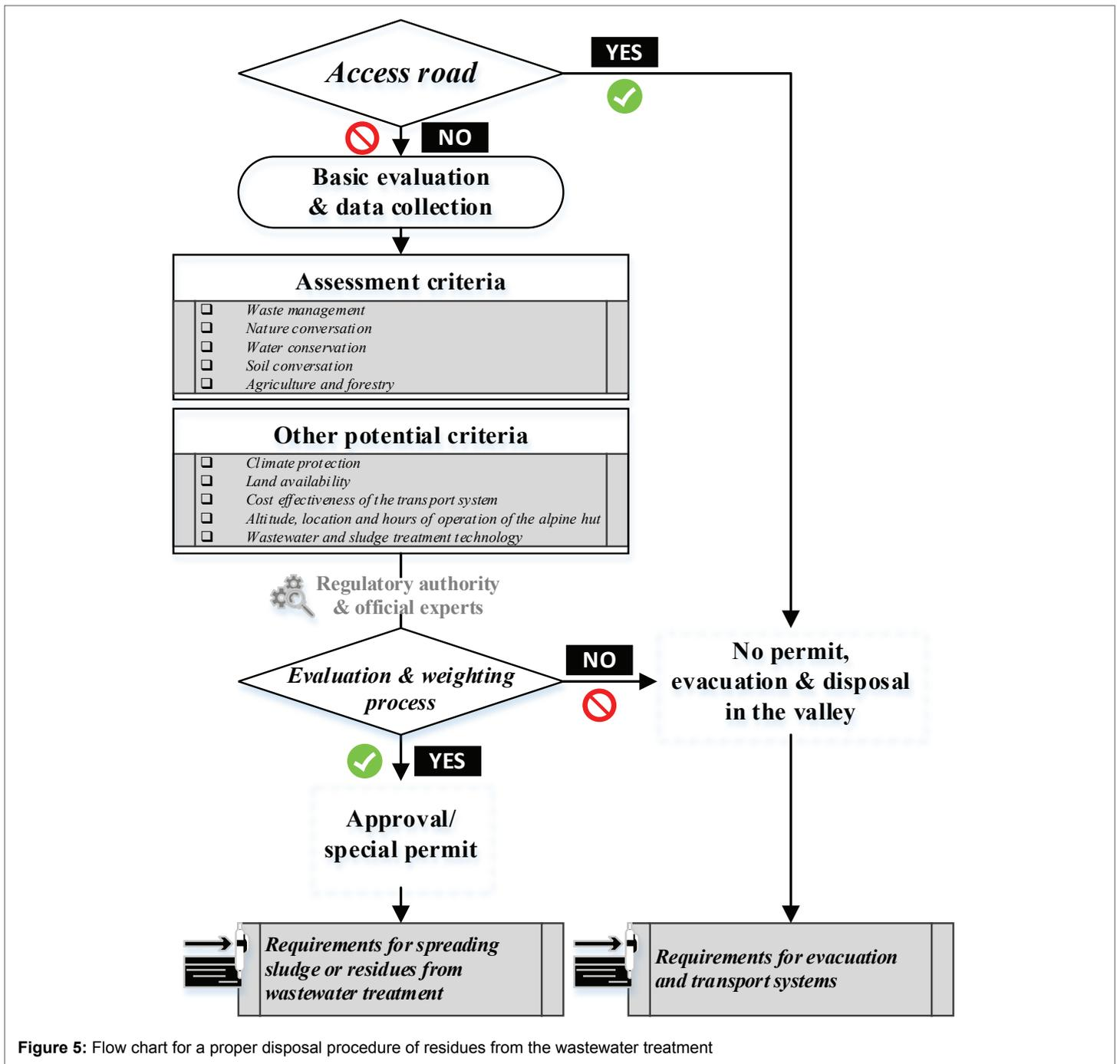
Figure 5: Flow chart for a proper disposal procedure of residues from the wastewater treatment
