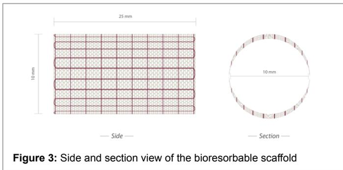
**Figure 3:** Side and section view of the bioresorbable scaffold
