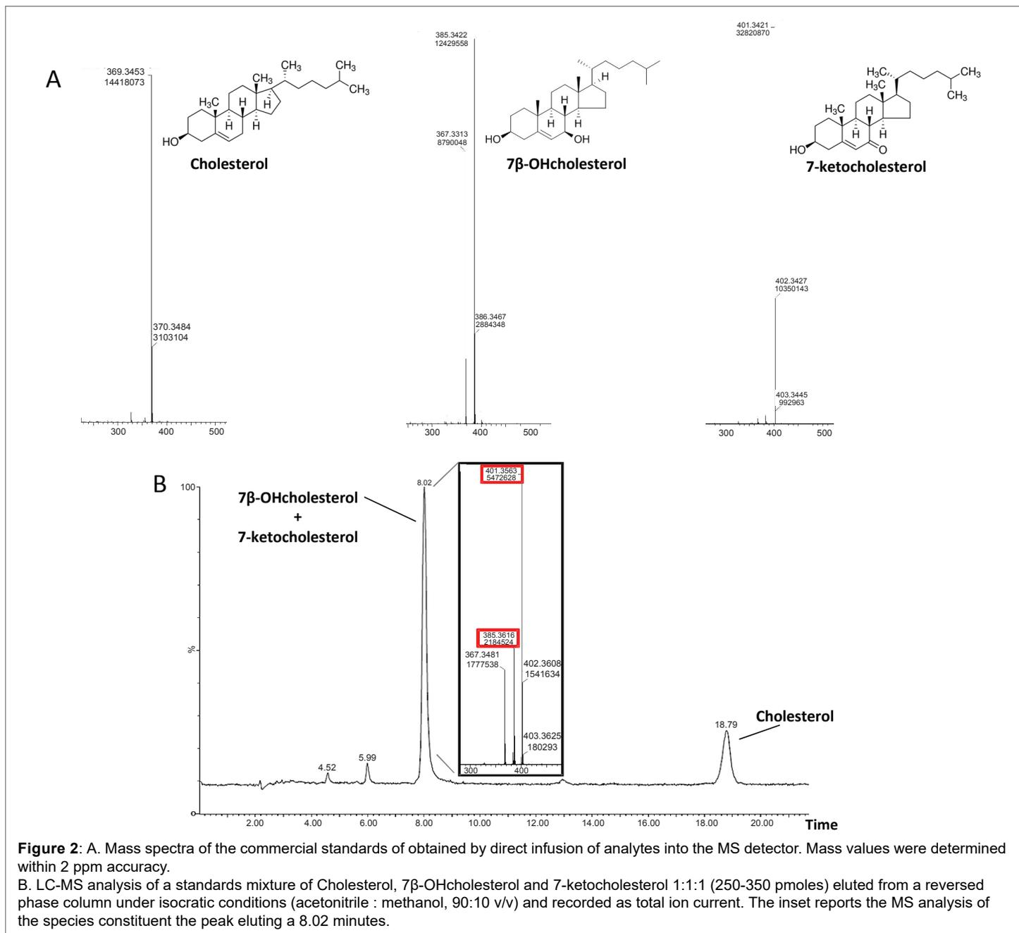
**Figure 2:** A. Mass spectra of the commercial standards of obtained by direct infusion of analytes into the MS detector. Mass values were determined within 2 ppm accuracy.
