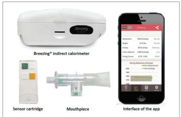
**Figure 1:** The Breezing® indirect calorimeter, sensor cartridge, mouthpiece, and iPhone interface of the application [10].
